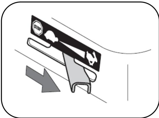
4. Firmly hold the handle of the recoil rope; pull the starter cord slowly until resistance is felt, then pull rapidly as shown in Fig. below.
