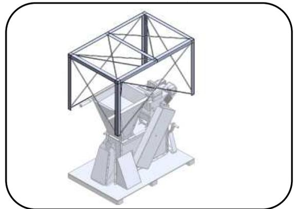
4. Remove the chipper by unscrewing the shipping fasteners. See figure below.
